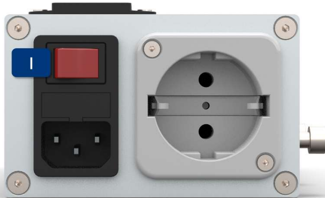
Figure 18 - Electronics box of the alarm unit; front surface
